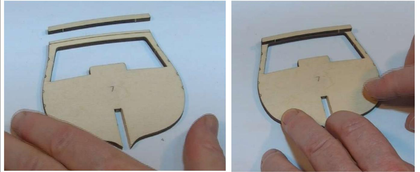
**Step 4** Identify the rear main deck supports 14 - fit and glue the part in place between the score lines on bulkhead 10 as shown.
