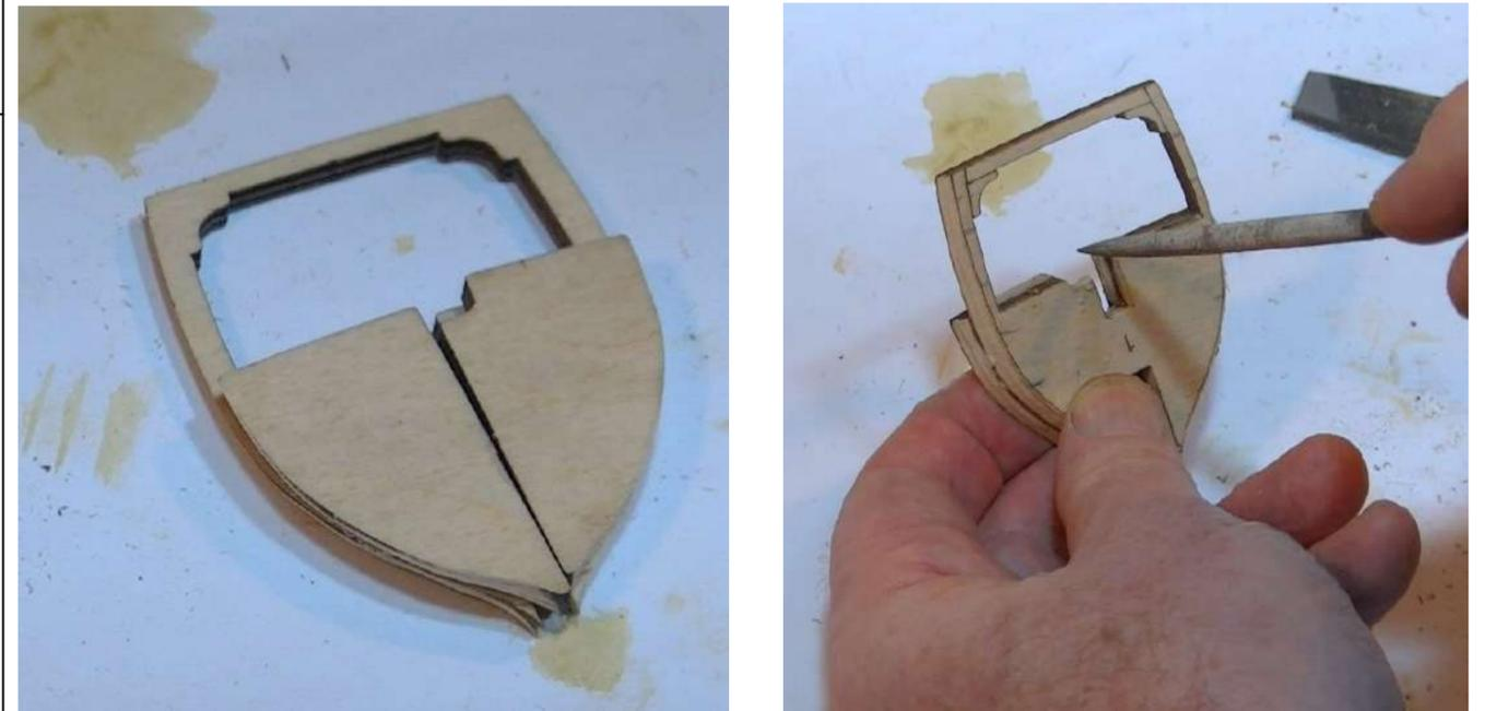
**Step 5** Trial assemble and then glue together the bow blocks 15C-F as shown. Set the glued bow blocks aside to be fixed in place later.
