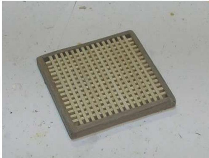
**Step 6** identify the hatch cover P49. Cut lengths of 2x3mm walnut P48 to make a frame as shown. File the frame to be flush with the cover. Stain the cover teak. Set aside to be fitted to the deck later
