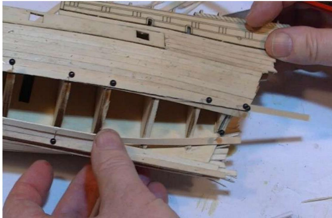
**Step 10** Continue the process of straightening the run of the planks previously presented to progressively close the remaining gap.
