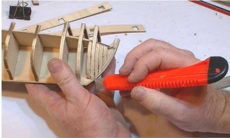
**Step 17** Place short lengths of sticky tape over the outside face of the horns on bulkheads 4, 5 & 6 - this will ensure the bulwark is not glued to the horns and will allow for the easy removal of the horns later. Take the bulwarks and trial fit between bulkhead 1 and bulkhead 9. Once satisfied glue, pin and clamp in place as shown.
