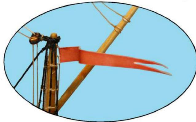
**Orange Streamer P126A** - tie lanyard off at the top of the mizzen mast and to the mizzen at the base of the streamer.
