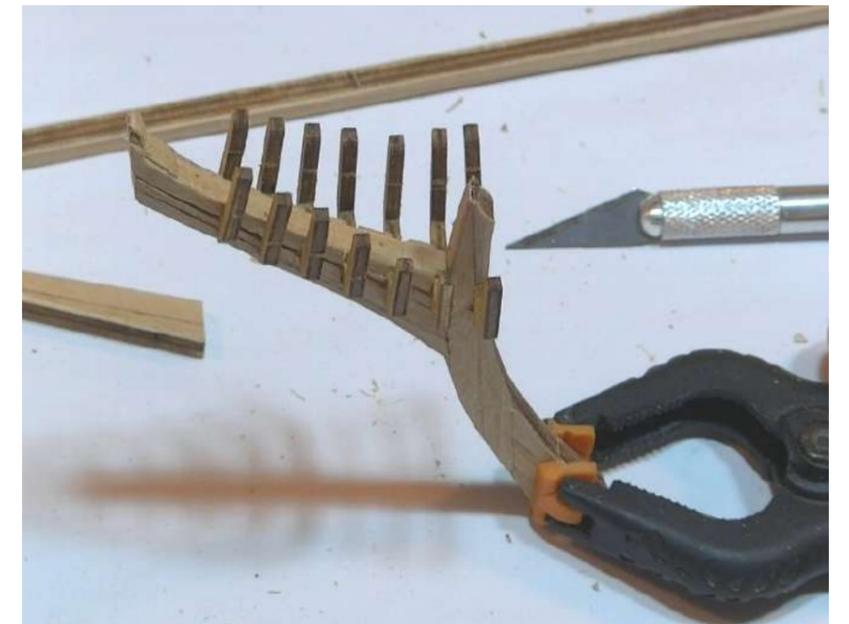
**Step 13** Trial fit the assembled stem post - once satisfied use a two part 5mm epoxy glue to fix the stem post in place - pin in place until glue has set as shown. Glue and pin the stern post in place as shown. Glue and pin in place the false keel as shown. Finally give the completed hull a sand with a fine grade sandpaper.
