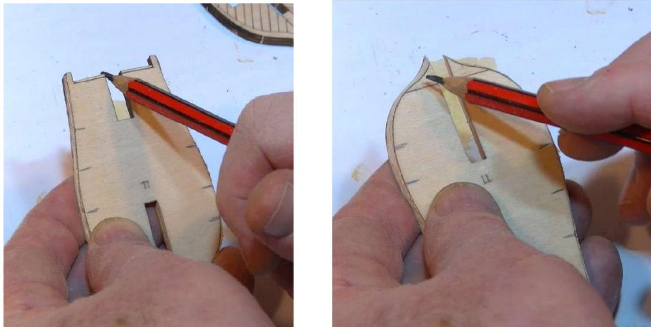
**Step 3** Identify the bow filler blocks P15A-F. Fair each of these parts from the score line to the other edge as shown.
