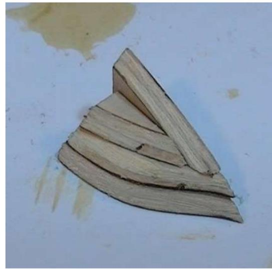
**Step 6** Identify the main deck pieces 16A-D - apply a few coats of shellac to the decks - allow to dry between coats.
