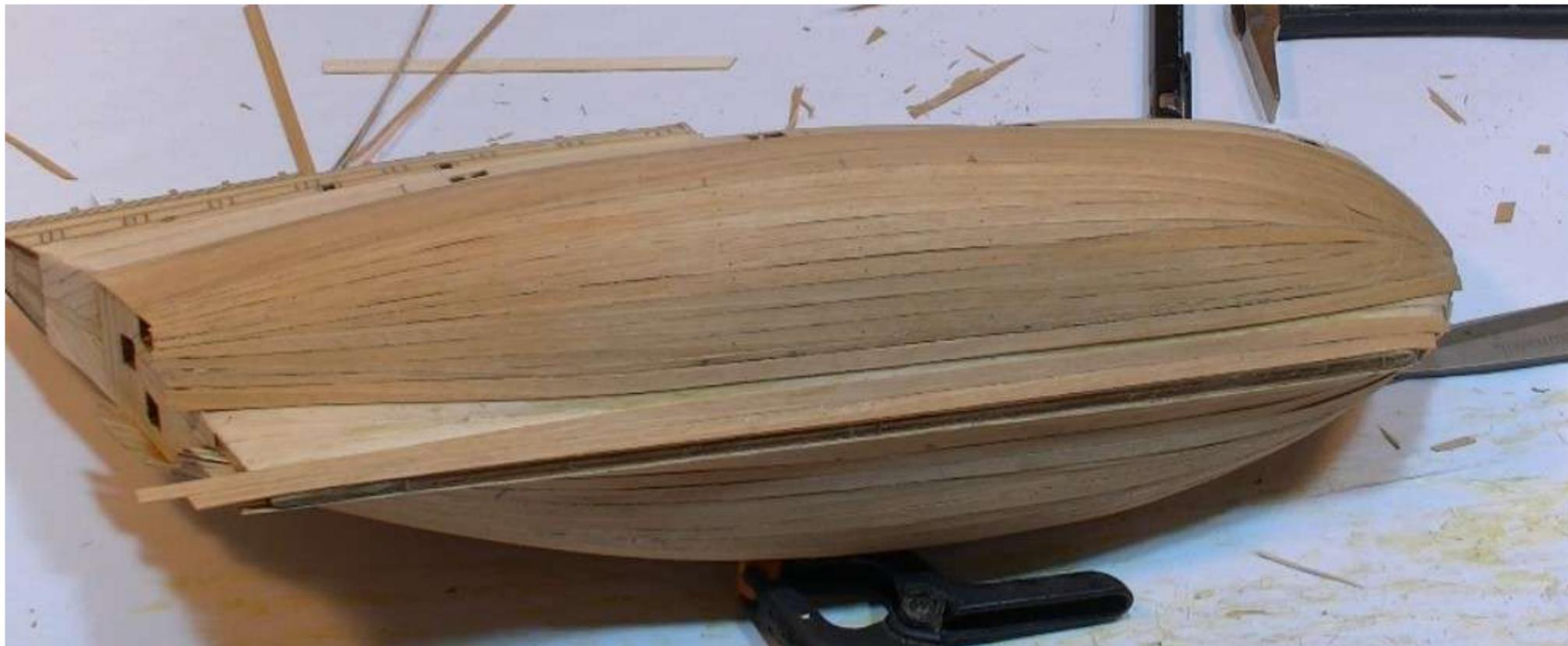
**Step 4** The remaining gap may be slightly less than 4mm from the mid-ship area to the bow. Lay a plank over this area as shown - mark the area of overlap with the upper plank then use a knife to remove the unwanted plank length - this will leave a 4mm wide gap in which to fit the last plank. Glue this plank in position. Close the deadwood area up with wedges.
