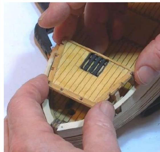
**Step 9** Cut lengths of 1x4mm limewood P25 to cover the side faces of the forecabin. Glue and pin in place as shown.
