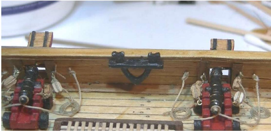
**Step 43** Identify the mast heels for the main mast P94 and mizzen mast P95 - file the upper rim round on each heel, stain teak and glue in position as shown.
