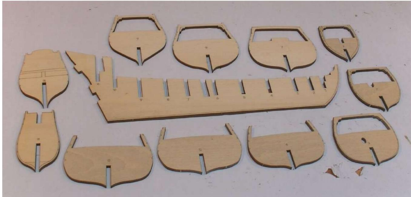
**Step 2** Dry fit the bulkhead frames into the keel slots. **Note: Bulkhead frame 11 is fitted with the number and score lines facing the rear.** Do not glue anything at this stage. Do not force the bulkhead frame into the keel slot. You may need to use a small flat file to fractionally open the slot in both the keel and bulkhead frame. The fit should be firm but no loose. Do not glue anything at this stage.
