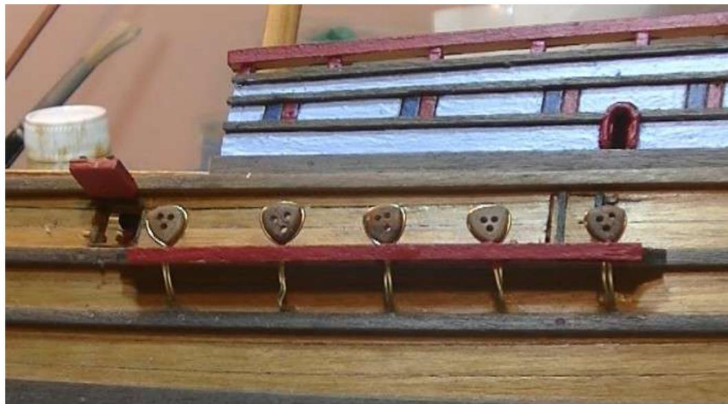
**Step 14 Gammoning block** - cut a 8mm length of 2x3mm walnut P48 as a block for the gammoning. Fix it in place on the bowsprit as shown. Use cord M for the gammoning - fit over the bowsprit and through the pre-cut slot in the stem post. Tie the gammoning together in the centre.
