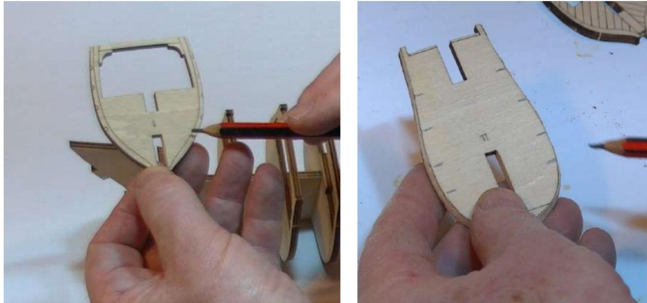
**Step 2** On bulkhead 11 file the top edge from the score line to the other face edge as shown. Also on this bulkhead at its lower edge file from the score lines to the other face edge as shown.
