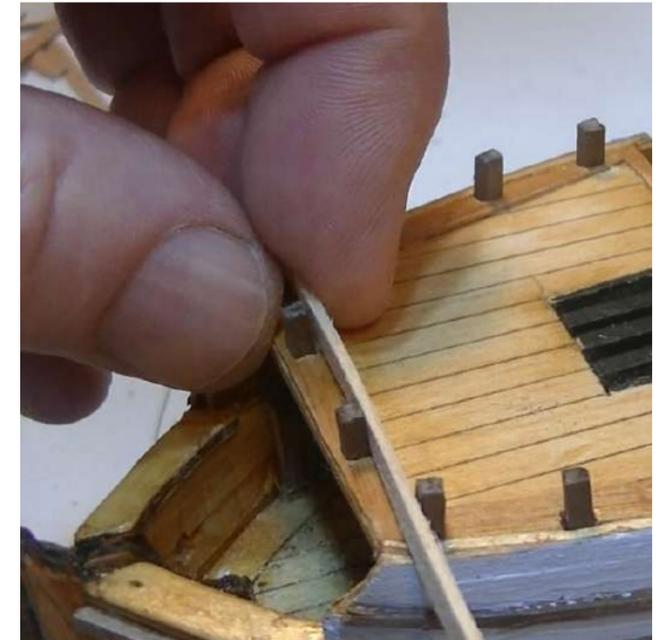
**Step 25** Identify the 1x2mm limewood P70 - fit and cut a length as shown - glue and pin and place - paint red as shown. Paint the forecastle posts red as shown.
