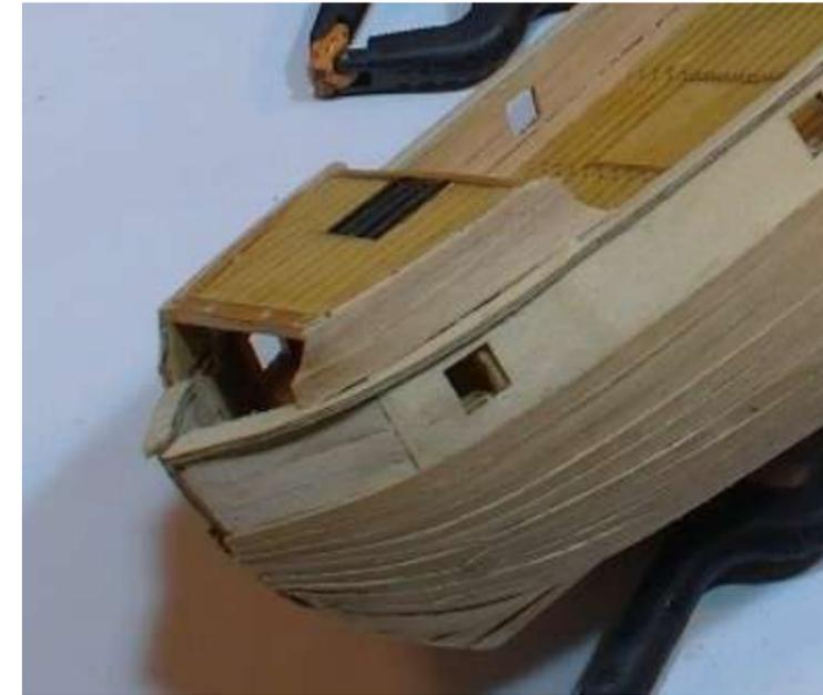
**Step 11** Use 4mm tanganka strips to complete the hull planking as shown. Cut out the gunports.
