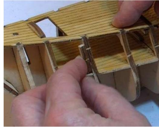
**Step 13** Identify the bulwarks P22A-B - note the port & starboard sides and the forward location - remove the gunport lids P23 and safely place away for use later. Trial fit the bulwarks in place. Fair the bulkhead frames and deck edge to accommodate the bulwarks. Fractionally adjust as necessary.
