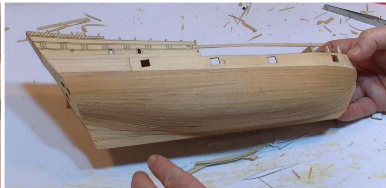
**Step 5** Use a knife to cut through and remove the bulkhead horns exposed on the main deck. Glue tangenika strip in place along the edge to cover the exposed bases. Also lay tangenika strip along the outer edge of the poop deck as shown. Glue in place tangenika strip on the inside face of the bulwark on the main deck - mark and cut-out the gunports.
