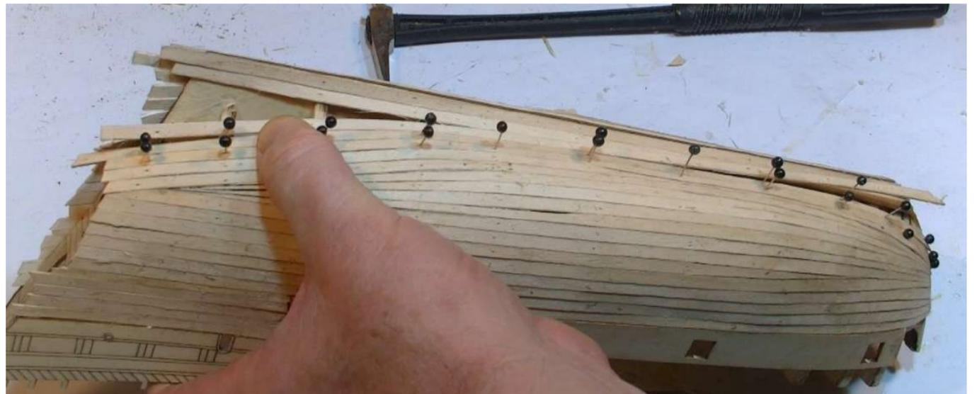
**Step 13** Cut triangular wedges to progressively close-up the gap in the deadwood area as shown. Glue and pin wedges in place.
