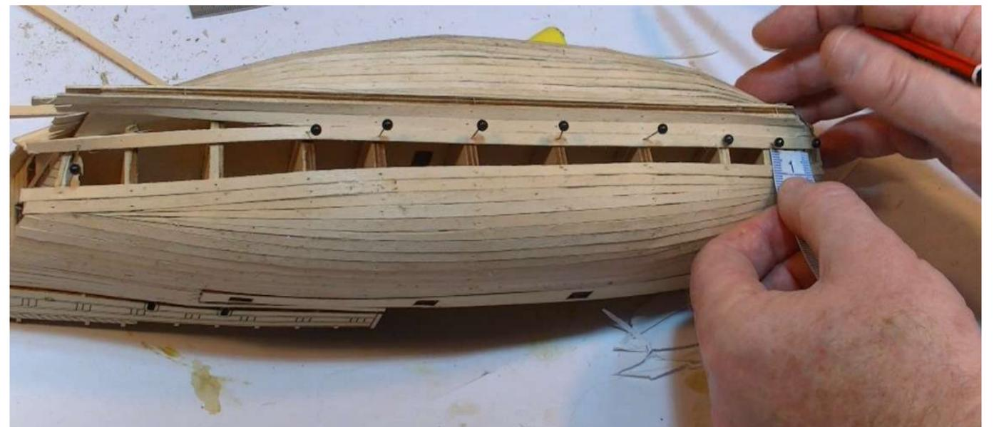
**Step 12** Lay a temporary guide plank over the last plank fitted and along these marked 8mm points - pin the plank in position and mark the area of overlap. Cut the area of overlap away. Remove the temporary guide plank. Remove the temporary plank fitted at Step 7 and now glue and pin this plank back in place. Glue and pin two planks in place to fill the remaining gap.
