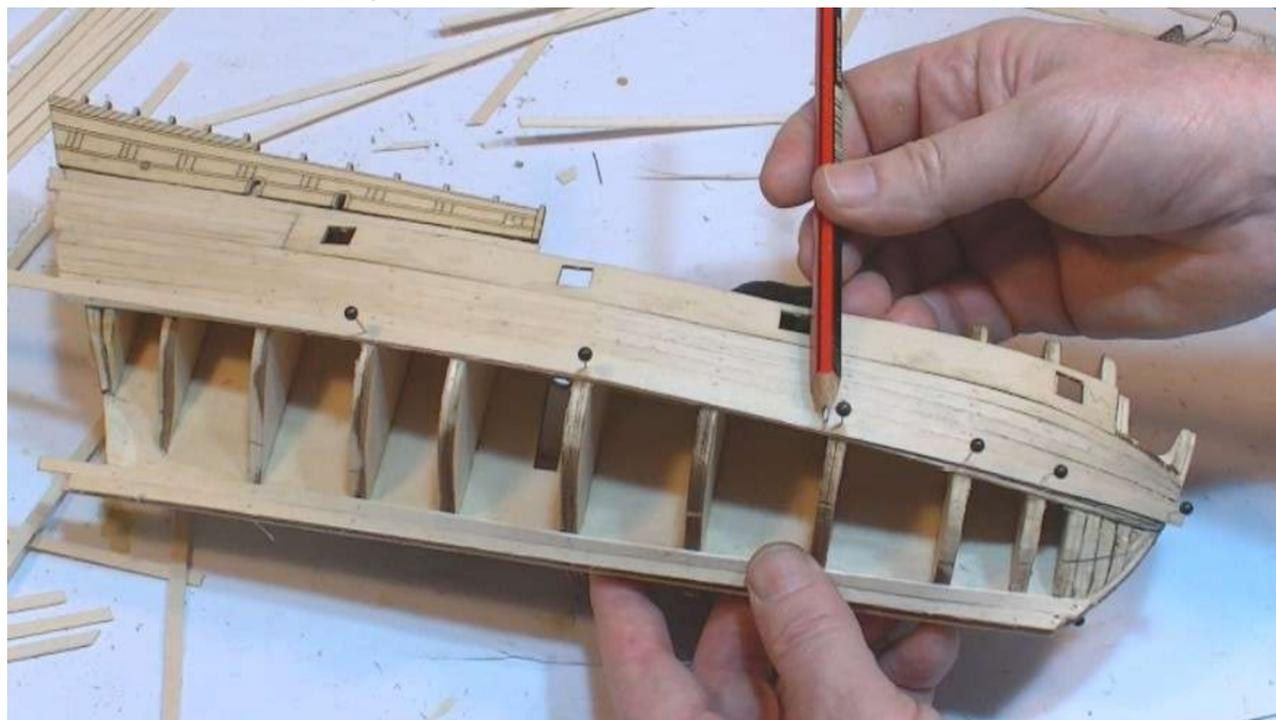
**Step 7** Temporarily pin a plank in place across the mid-ship bulkheads 5 to 7 immediately adjacent to the planks at the keel as shown. Pin the plank in place at the junction of bulkhead 11 and the transom base as shown. At the bow pin the plank in place adjacent to the 2nd plank from the keel.
