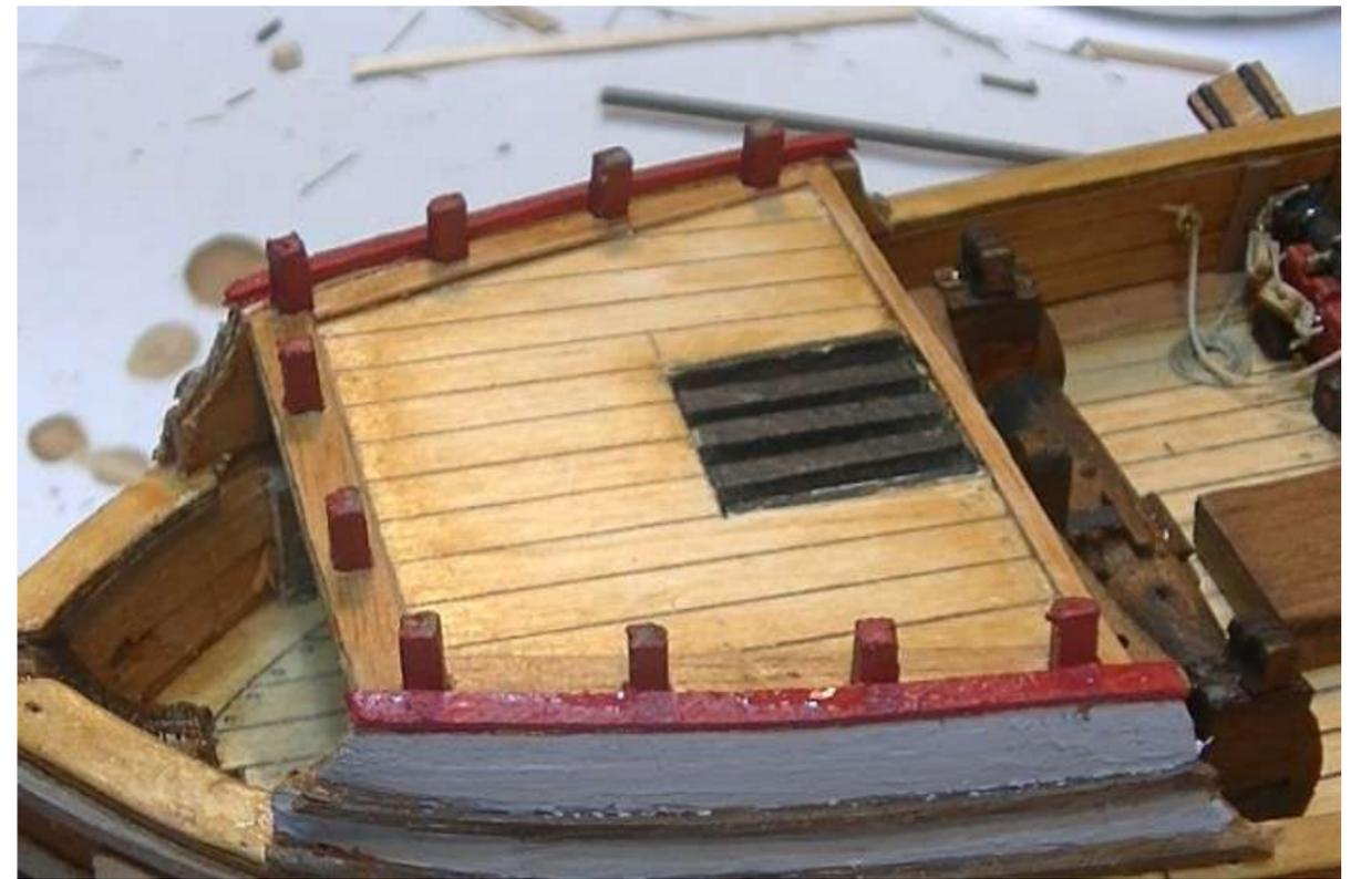
**Step 26** Identify the forecastle cap rails P71 - trial fit in place - fractionally adjust as necessary - once satisfied glue in place as shown. Identify the bitt heads P72 - glue in place as shown. Paint the cap rails and bitt heads red.
