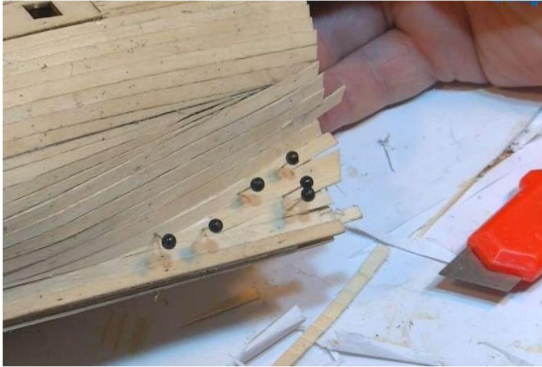
**Step 14** To complete the first layer of planking fit, shape and glue in place lengths of limewood planking between bulkhead 1 and the stem post as shown.
