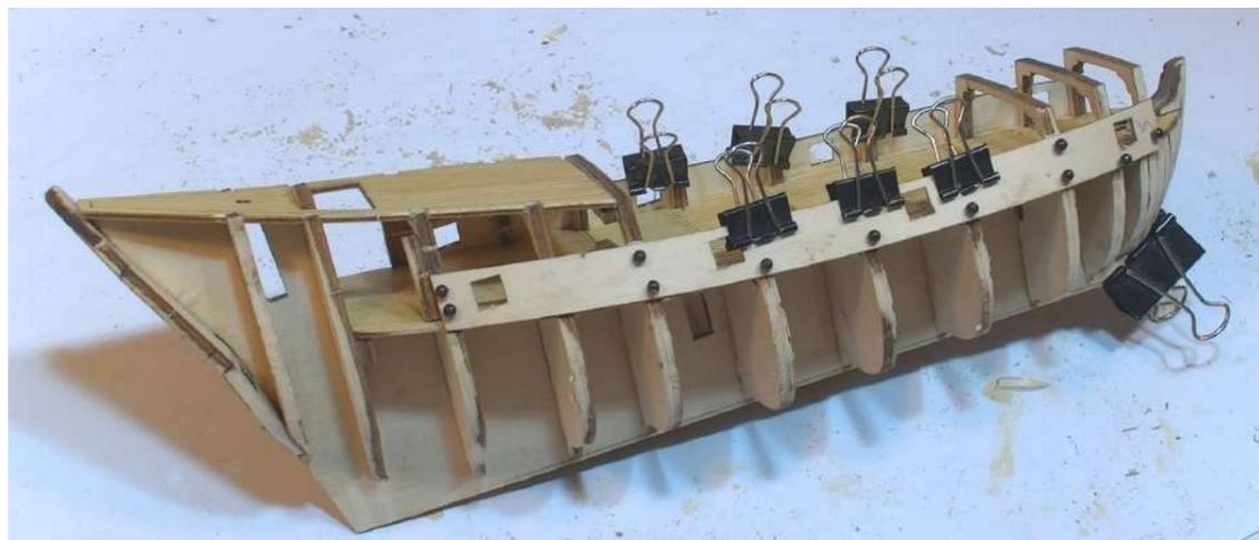
**Step 18** Identify the 1x4mm limewood timber strips P24. Take one length and pin in place at bulkhead 7 immediately above the bulwark. Identify the side panels P26 - trial fit one in place aligning the rear edge with the top of, and at same angle as the transom. The front lower edge of the panel is to lay on the plank as shown - once you are satisfied with the alignment glue and pin the panel in place as shown.
