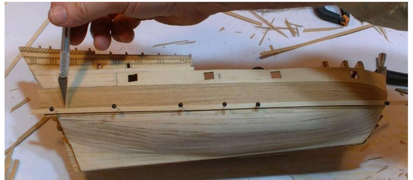
**Step 3** Continue the process of planking and making corrections using a limewood plank as a guide to mark the area of overlap and remove the unwanted planking. Continue until you start to close around the lower section of the hull as shown - fit the garboard plank and one plank adjacent to the garboard as shown.
