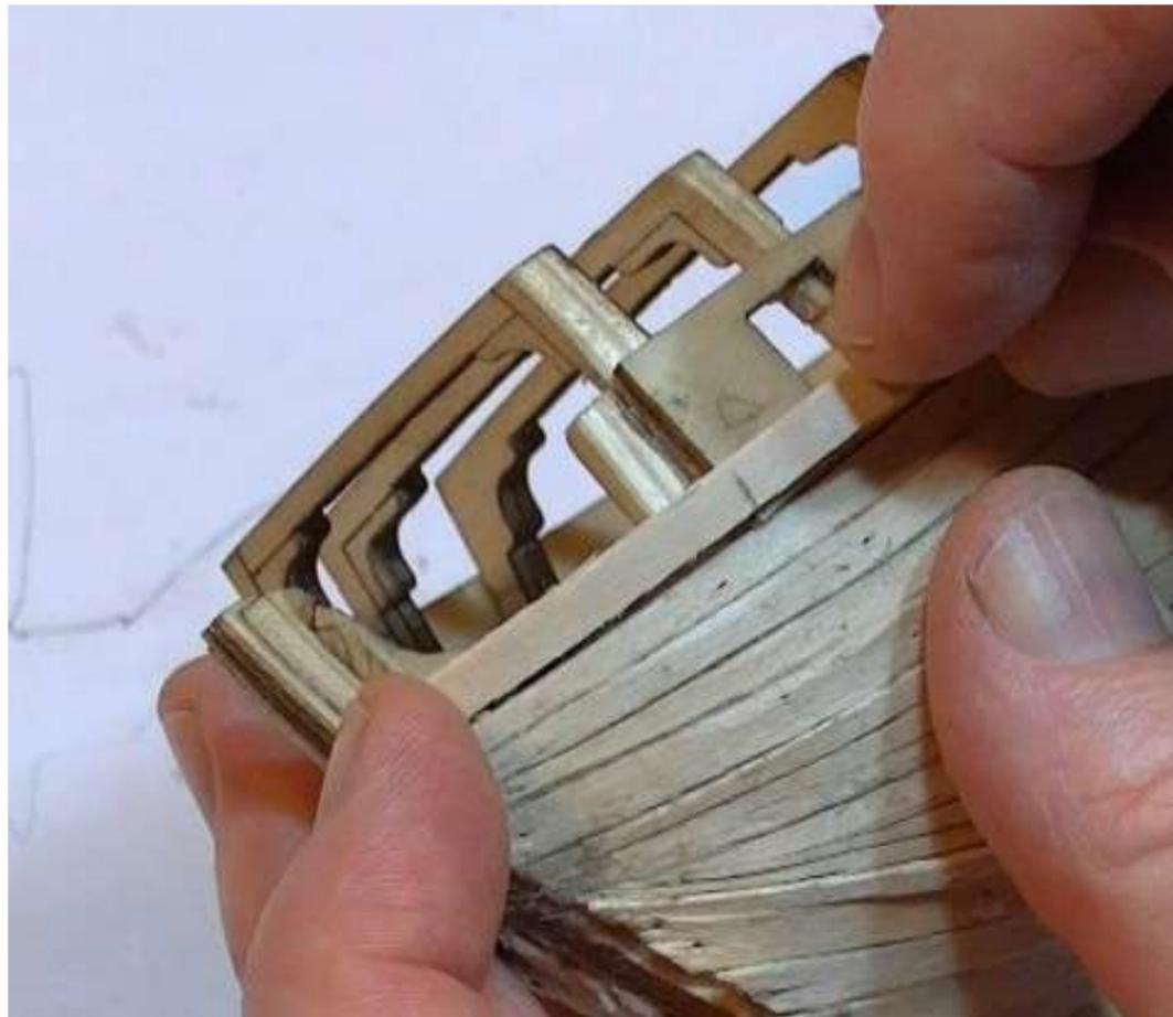
**Step 15** The first layer of planking is now complete. Next trim-off any excess planking at the stern area. Then use wood filler to fill-in any gaps between planks and give the hull a thorough sanding until the hull is perfectly smooth.
