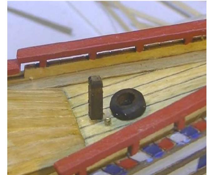
**Step 44** Identify the anchors P92 - assemble as shown. Cut 2 x 250mm lengths of 2mm cord P93 - seize the cord around the anchor ring as shown. Lash the anchors to the top head rails as shown. Feed the anchor rope through the hawse holes, wind around the windless as shown and feed ends into hawse pipes on the deck.
