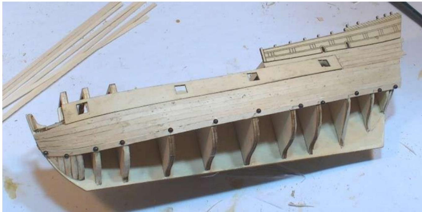
**Step 5** Next fit and fix in place the garboard plank - this plank is not tapered. The garboard plank is fitted along the length of the keel as shown - trial fit and once satisfied glue and pin in place. Glue and pin a second plank immediately adjacent to garboard plank as shown.
