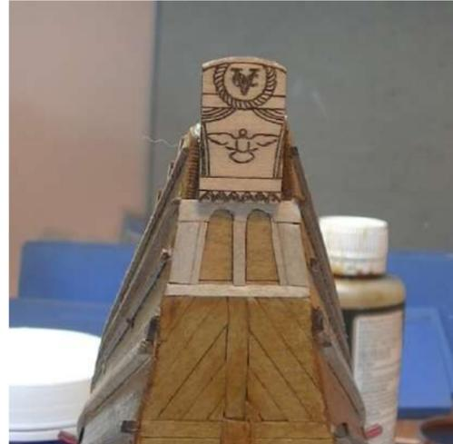
**Step 21** For the flag support identify the 3x3mm limewood P66 - cut a length to 15mm. Cut a 7mm length of 2x3mm walnut P48. Shape the top end of the limewood so that the walnut piece sits horizontal as shown. Once satisfied glue each part in place as shown.
