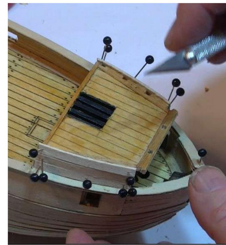
**Step 10** Identify the forecastle fillets - rear P34 and fore P35. Trial fit in place as shown and fractionally adjust as necessary - once satisfied glue each part in position. Use 4mm tanganka strip P29 to cover the forecastle sides and fillets as shown.
