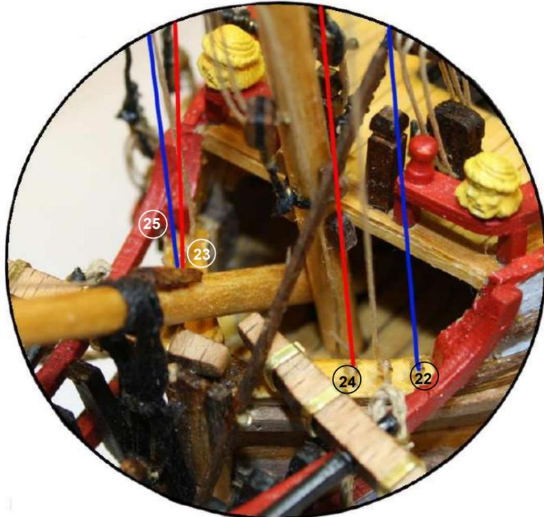
**Step 36 Belying Pins** - Identify the belying pins P125 - fix to the belying locations on the main deck, winch and bowsprit as shown.
