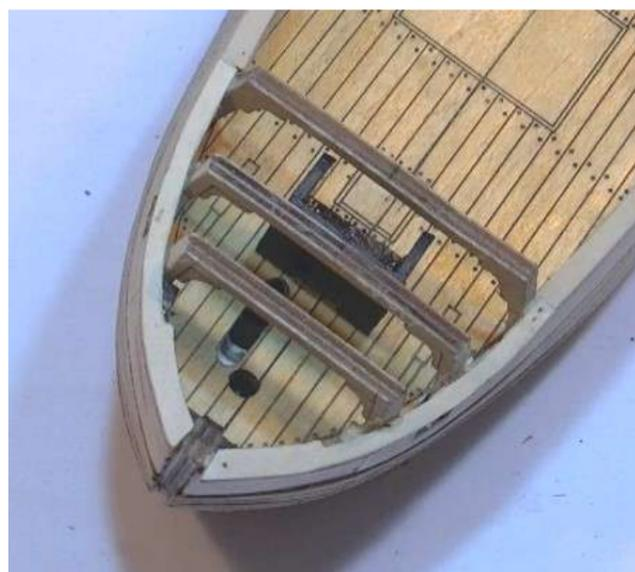
**Step 8** Identify the forecabin deck P33. Fit 4mm tangenika strip P29 on the side and fore edges. Cut a length of tangenika strip to 2mm width and fit to the rear edge. Use a square needle file to open and shape the slots. Apply shellac to the deck and tangenika strips. Paint the stove grating black as shown.
