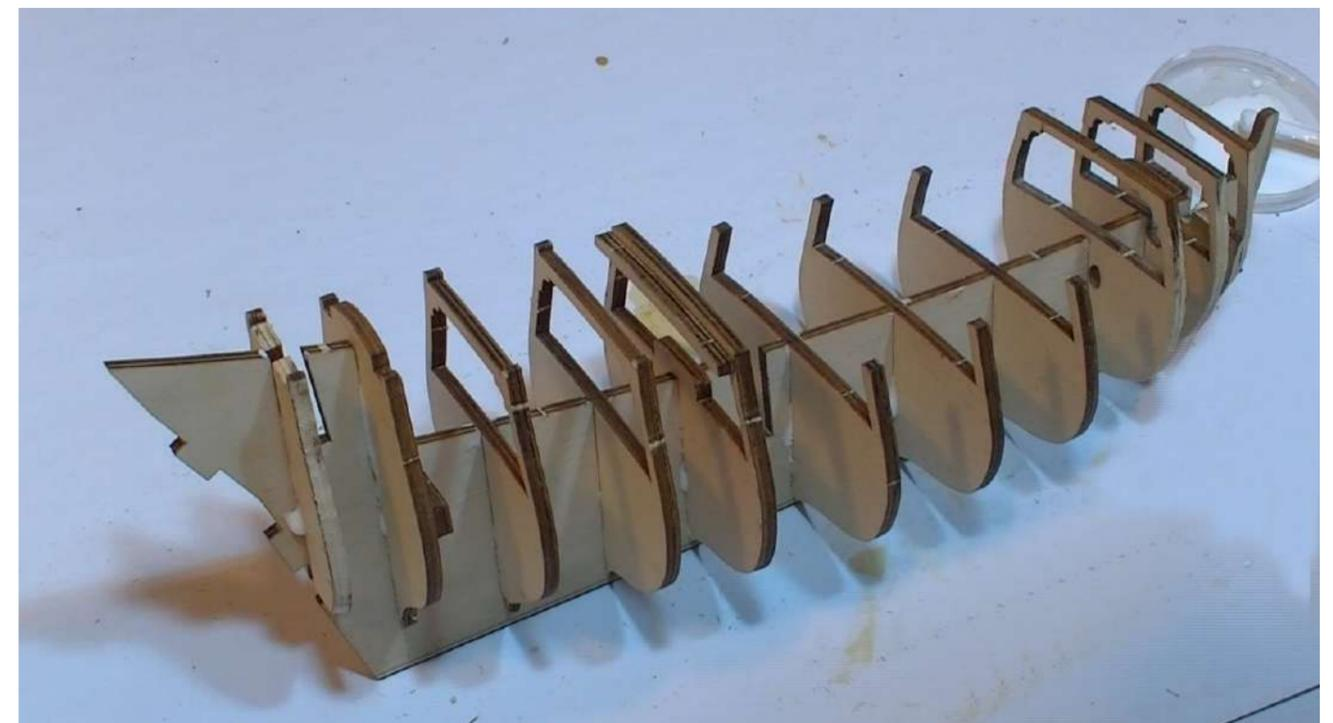
**Step 8** Before the bulkhead glue as set apply glue to the top of the bulkheads and keel and fix in place the decks - use map pins to hold the main deck in place until the glue has set - this approach will hold the bulkheads square while the glue sets for the whole assembly. Set aside for 24 hours to allow the glue to fully set.
