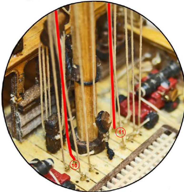
**Step 30 Lifts - Foremast - Fore Yard** Use cord K to rig the fore yard lifts as shown. Terminate at the belaying points 12 & 13 as shown. See also Sheet 56.
