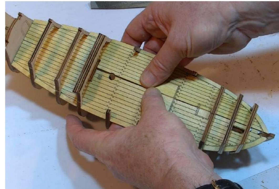
**Step 8** Glue the bulkheads in place as shown - remove any excess glue with a cotton bud.
