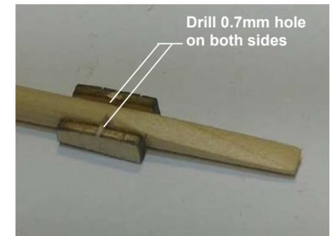
**Foremast - Upper** - Identify the 4mm dowel P103C - cut and shape as shown
