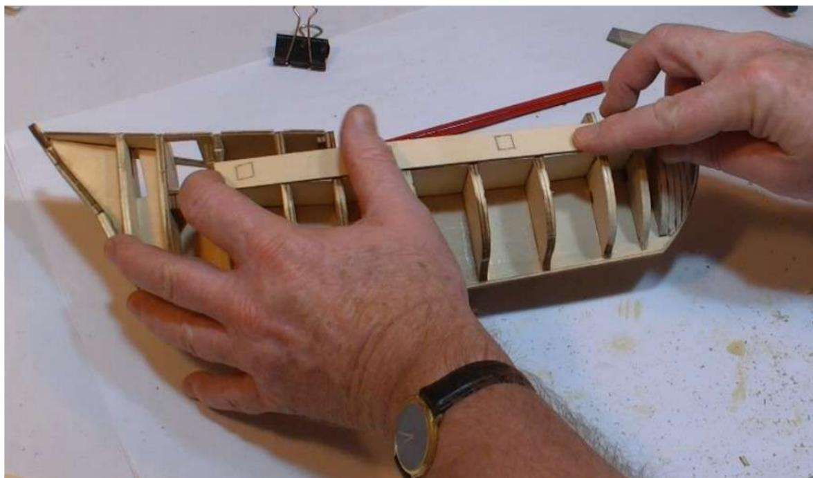
**Step 14** Fairing - complete the fairing process by using a plank to check across the bulkheads to ensure where the plank rests on the bulkhead it will be full face on to the bulkhead. Fractionally adjust using a flat file where there are edges. Continually check and adjust as necessary.
