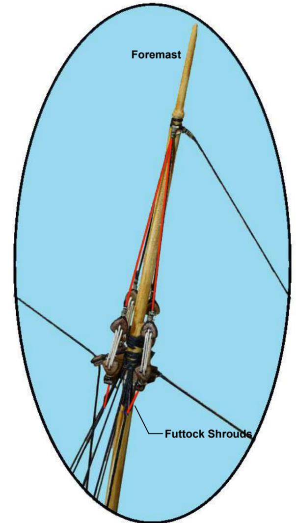
**Step 21 Backstays - Main Mast and Foremast** - for each pair of backstays cut a length of cord M long enough to go from the topmast down to the cap rails as shown. Seize the cords together at the topmast as shown. Fit block D to each end of the cord. Reeve the blocks together using cord K starting at the eye pin previously fitted to the lower block and terminating on the stay immediately above the upper block as shown.
