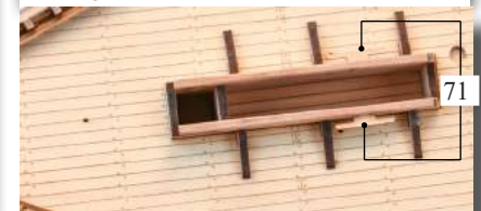
Above - Add part numbers 39, the Fore Mast Opening Side Checks. Slot and glue into place as shown above and left. Below - Slot and glue the cleats (71) in place on the outside all of the fore mast housing sides.
