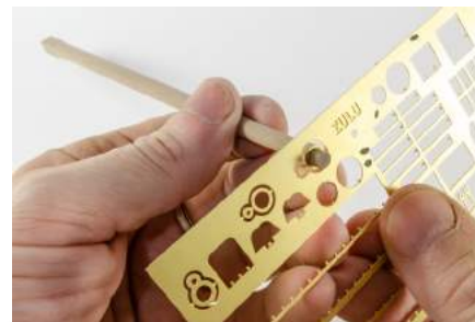
Above - Tapering can be gauged by slotting the mast rings in place. Once it fits tightly, the taper is enough.
