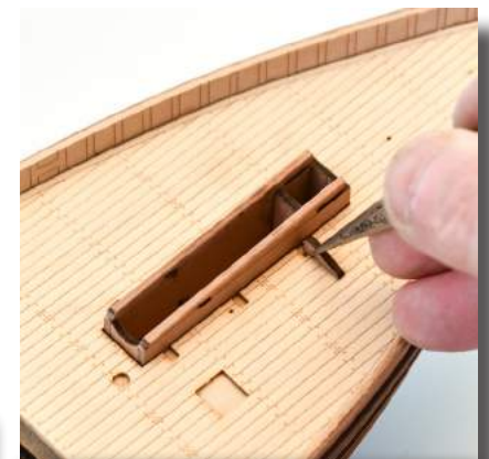
Above - Add part numbers 39, the Fore Mast Opening Side Checks. Slot and glue into place as shown above and left. Below - Slot and glue the cleats (71) in place on the outside all of the fore mast housing sides.
