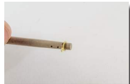
Above - End of fore mast showing mast ring and the 1mm holes for the fore and main sail lifts.
