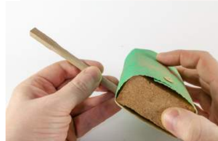
Above - Tapering the fore mast, note that the foot of the mast is left square.
