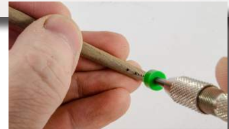
Above - Drilling the 2 holes near the top of the fore mast, as shown in the plans.
