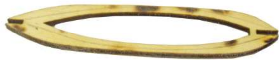
Step 4 Shape layer 2 from the pencil line as shown. Turn the layer over and shape internally from the score line to the internal cut line as shown.
