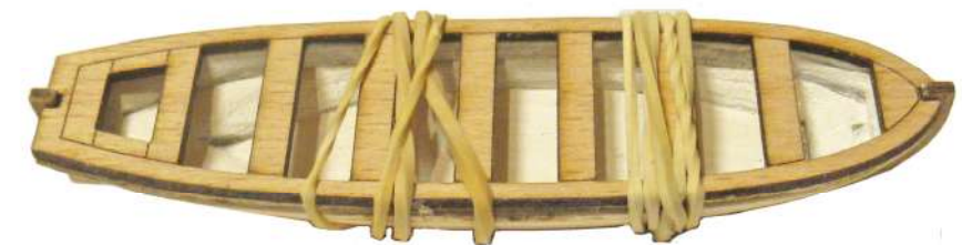
Step 11 Sand the hull to ensure a smooth transition between layer. Use a water moistened wood filler to fill any gaps.
