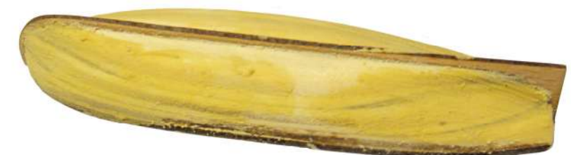
Step 11 Sand the hull to ensure a smooth transition between layer. Use a water moistened wood filler to fill any gaps.
