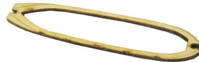
Step 7 Shape layer 3 from the pencil line as shown. Turn the layer over and shape internally from the score line to the internal cut line as shown.
