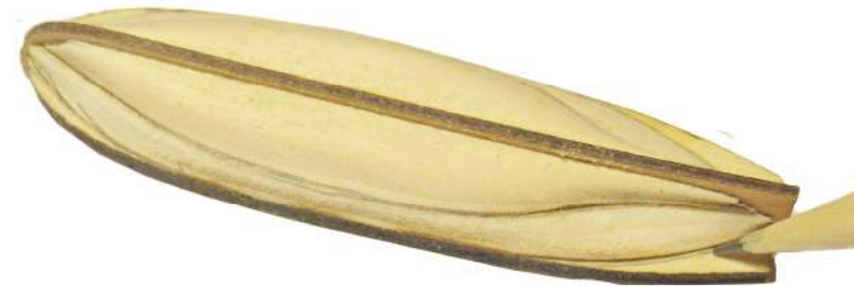
Step 7 Shape layer 3 from the pencil line as shown. Turn the layer over and shape internally from the score line to the internal cut line as shown.
